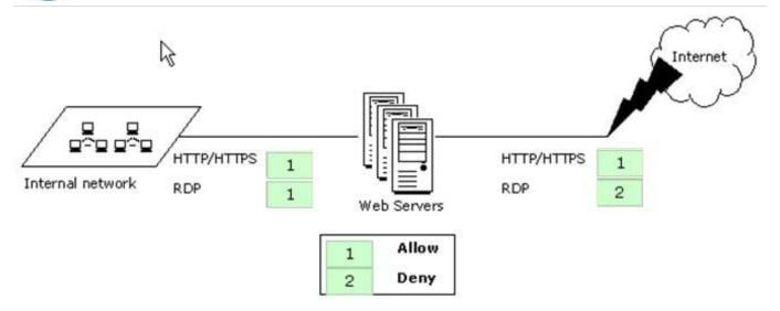
HTTP/HTTPS is used for transferring HTML pages over the network. Hence, you should allow it for both the Internet and internal clients traffic.
