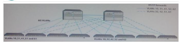
The exhibit shows a network with HP 3500 yl Series switches at the access layer and HP 8206 zl switches at the core. The customer with this solution has logged several support calls, which were eventually tracked down to spanning tree issues. How can a network architect adjust the solution to prevent the issue in the failure?
