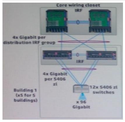
A network architect has designed the topology shown in the exhibit. The Gigabit links between distribution layer and the core uses OM3 grade multi-mode fiber between 100m and 150m long.
