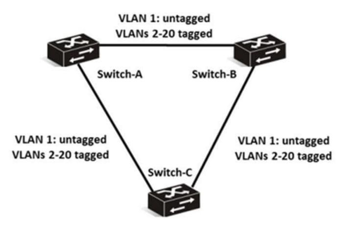
A network administrator has created a Layer 2 network based on the design shown in the exhibit. Switch-A and Switch-B are distribution layer switches. Switch-C is an access layer switch. All switches are HP Comware switches.
