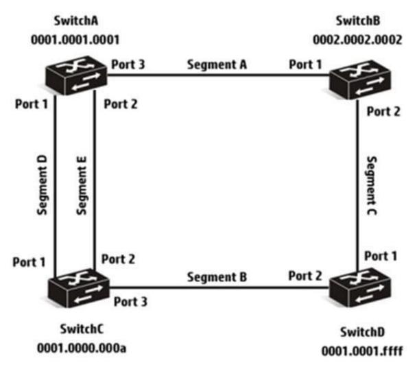
Assume the network shown in the exhibit has implemented RSTP Based on the topology, which port is a root port?
