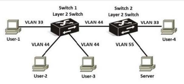
Switch 1 and Switch 2 are HP ProVision switches operating as Layer 2 switches. VLAN 33 has been defined as the management VLAN on both switches. Based on this topology, which user devices can access Switch 1 by using SSH?
