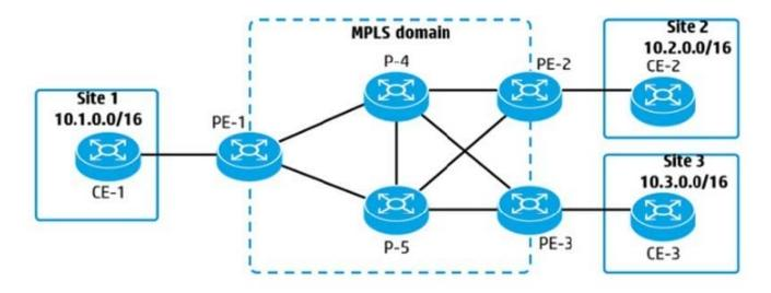
An administrator is planning an MPLS solution and wants to make sure that traffic from 10.1.0.0716 to 10.2 0.0/16 takes the best path. The solution is not using Traffic Engineering (TE). How does PE-1 choose between the label advertised for 10.2.0.0/16 by P-4 and by P-5?
