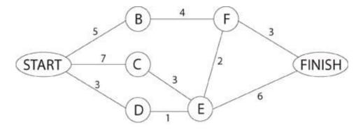
Which of the following is the float of path Start-C-E-Finish in the network diagram?
