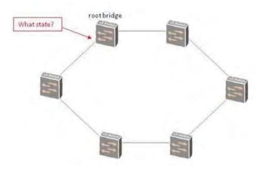
Based on the exhibit, in which spanning-tree state would the indicated port be?
