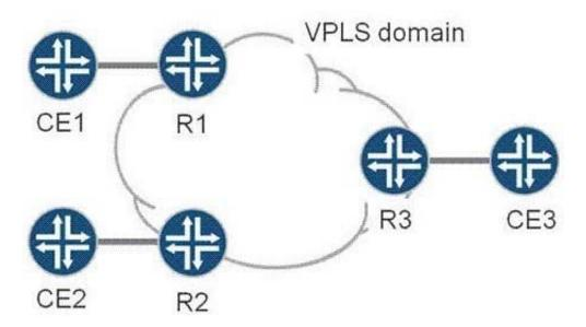
CE1, CE2, and CE3 are part of a single VPLS VPN. R1, R2, and R3 are PEs in the provider network, and have just been powered on. The VPLS domain has converged, and frames have passed between all CEs in the last minute. An Ethernet frame has just arrived at R3 from CE3. It has a source MAC address of CE3 and a destination MAC address of CE1. What does R3 do with the Ethernet frame?
