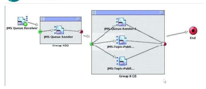
This process uses JMS Local transaction. The JMS Topic Publishers all point to JMS Shared Connection1. The JMS Queue Senders all point to JMS Shared Connection2. The JMS Queue Receiver is configured to tie into Group A(1).
