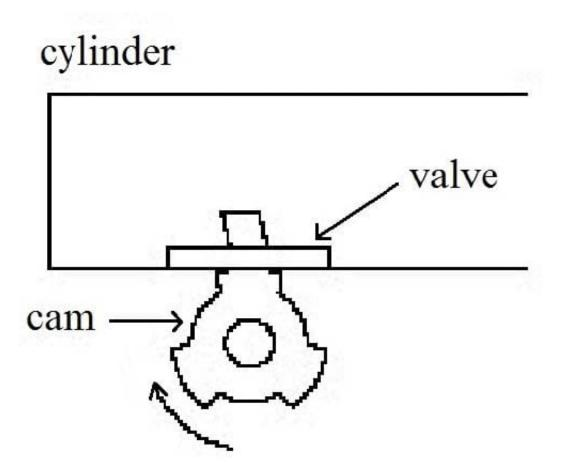
In the figure above, for each complete revolution the cam makes, how many times will the valve open?
