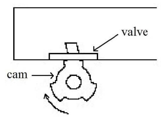
For the valve shown in the figure above to open once each second, the cam must revolve at a rate of \_\_\_\_\_\_
