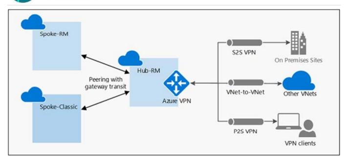
In the diagram, gateway transit allows the peered virtual networks to use the Azure VPN gateway in Hub-RM. Connectivity available on the VPN gateway, including S2S, P2S, and VNet-to-VNet connections, applies to all three virtual
