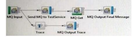
A second application, namedTestService, contains the message flow that processes messages sent from theSend MQ to TestServiceMQ Output node and returns the response message that is then retrieved by the MQ Get node. This application is already deployed to the Integration Server that is nameddefault.
