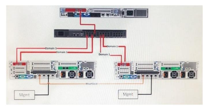
Based on the exhibit, a customer is using Virtual Port Mode. If the primary path for the controller on the "left" is disconnected while running an IOmeter test for a volume owned by the "left" controller, will the system survive failover?
