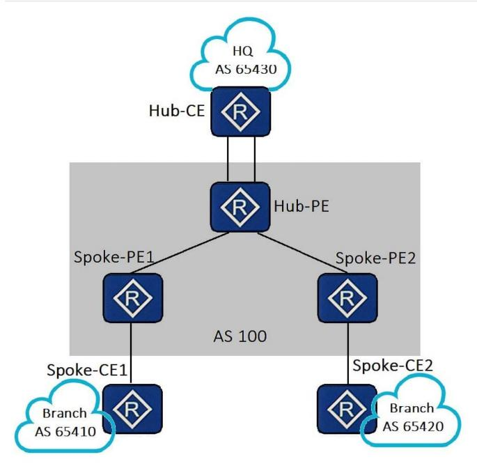
A. When the Hub-CE and Hub-PE use EBGP to transmit routing Information, the Hub-PE must be able to accept routes with the AS number repeated once so that routes advertised by the Hub-CE can be received.
