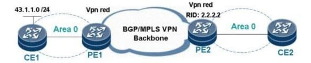
As shown in the figure, a CE requires access to the Internet, and PE 1 is connected to the Internet gateway. Configurations on PE 1 are as follows: PE 1: # nat address-group 0 175.31.1.3 175.31.1.10 # ip vpn-instance vrf1route-distinguisher 192.168.1.1:100
