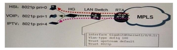
RTA is an edge route of the MPLS backbone network. It provides the access for users under layer 2 switches and differentiates user by subinterface. User access VALN 100 and has subscribed to the His ViIP, and services. According to 802 1p priorities, the value 0 indicates the HIS service, 1 indicates the Volp service and 4 indicate the IPTV service. The DiffSerc model is deployed in E-LSP mode on the MPLS network,
