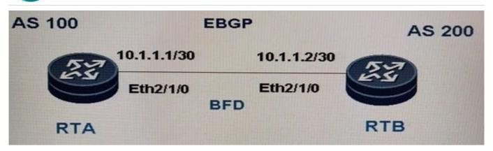
As shown in the figure, RTA and have one BGP session. To detect fault fast, the BFD for BGP feature needs to be configured on RTA and RTB. BGP-related configurations are as follows:
