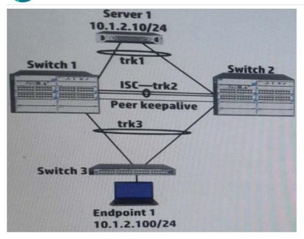
Switch 1 and Switch 2 have established and Interswitch Connection (ISC) and two distributed trunks. All of the switches have Multiple Spanning tree Protocol (MSTP) enabled. Where does Switch 1 transmit or process Bridge Protocol Data Units (BPDUs)?
