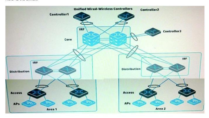
A company has two HP Unified Wired-Wireless controllers. The MSM APs in Area 1 in the exhibit are controlled by Controller1. The MSM APs in Area 2 in the exhibit are controlled by Controlled. The company purchases a Controlled to provide backup for both Controller1 and Controller2 (N+1 redundancy).
