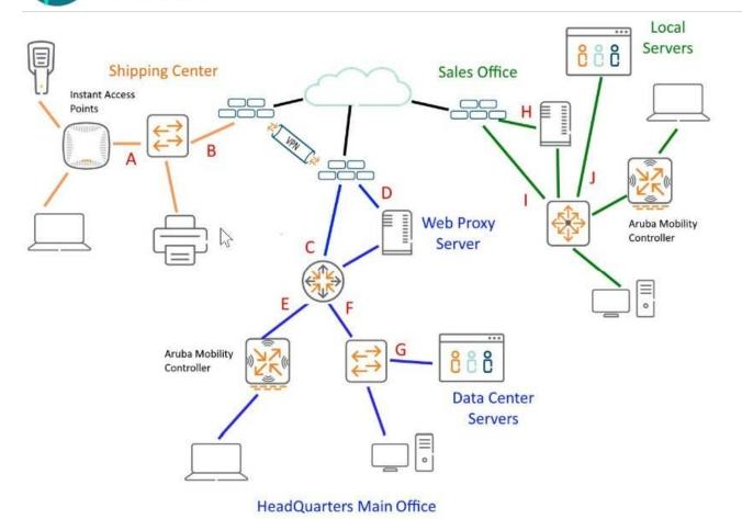
Given the network diagram, would this be a proper location for a network tap? (Port G at the Head Quarters Site would expose all East/West traffic bound for the data center.)
