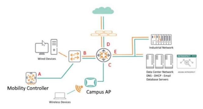
You are monitoring network traffic and considering DNS flow patterns. Where is a good location to place the Network Tap or Taps? (Location C.)
