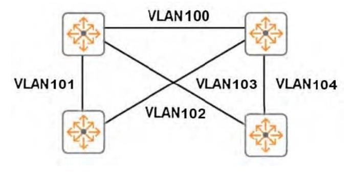
The switches in the exhibit are all ArubaOS switches that run MSTP. The network administrator wants all of the switch-to-switch links shown in the exhibit to be available for forwarding routed traffic.
