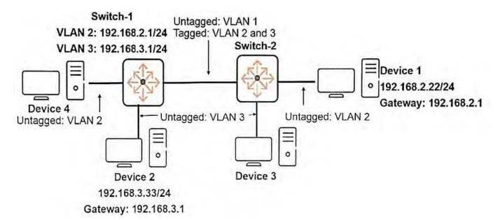
Device 1 needs to send traffic to Device 2, and it sends an ARP request in preparation. Which devices process this ARP request?
