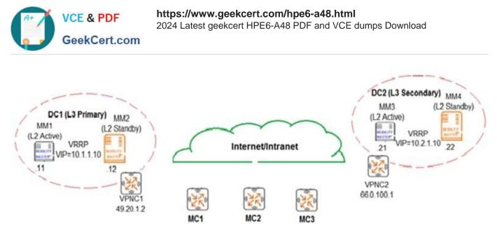
An Aruba network is deployed with L2 and L3 Mobility Master (MM) redundancy across two datacenters, as shown in the exhibit. The network administrator confirms that all Mobility Controllers (MC) are currently communicating with MM1, which is the L2 Active, and L3 Primary. Which MM IP will MCs communicate with if MM1 fails?
