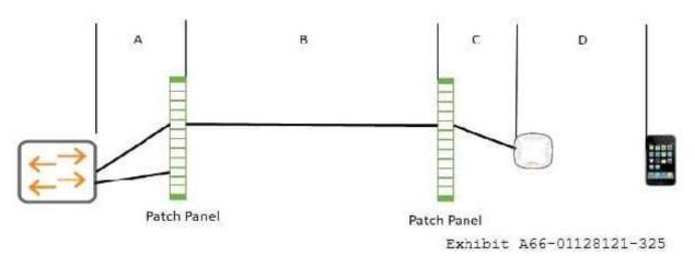
When planning the use of Cat7 cabling for a SmartRate connection between an ArubaOS AP and an ArubaOS switch, which sections should be considered when calculating distance?
