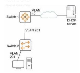
This company has ArubaOS-Switches. The exhibit shows one access layer switch, Swllcn-2. as an example, but the campus actually has more switches. The company wants to slop any internal users from exploiting ARP.
