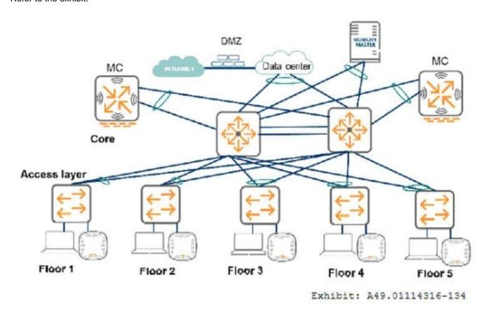
The exhibit shows the topology for a new Aruba solution. The MCs are in a ctuster and support all of the wireless traffic in
