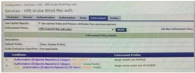
You have been asked to help a Customer troubleshoot an issue. They have configured an Aruba OS switch (Aruba 2930 with 16.09) to do MAC authentication with profiling using ClearPass as the authentication source. They cannot get it working.
