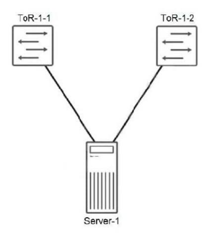
You are designing a data center where all your servers in each rack will be connected to two top-of-rack (ToR) switches using Layer 2, as shown in the exhibit. You must implement a high availability solution that maintains link layer connectivity to each server when one of the ToR switches fails.
