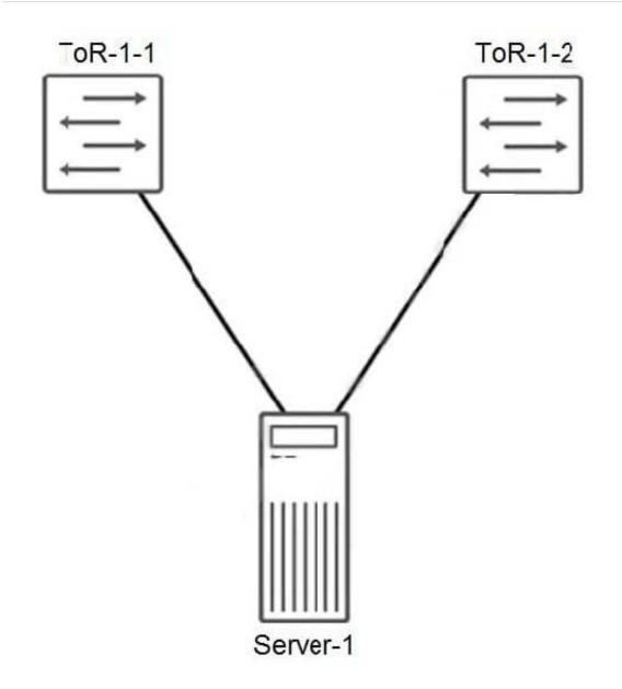
You are designing a data center where all your servers in each rack will be connected to two top-of-rack (ToR) switches using Layer 2, as shown in the exhibit. You must implement a high availability solution that maintains link layer connectivity to each server when one of the ToR switches fails.
