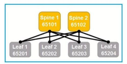
For a fully configured and functional IP fabric underlay as shown in the exhibit, how many external BGP neighbors are expected to be in established state for Leaf 1?
