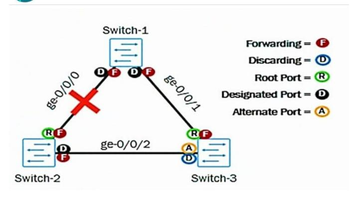
You manage the Layer 2 network shown in the exhibit. You experience a failure on the ge-0/0/0 link between Switch-1 and Switch-2.
