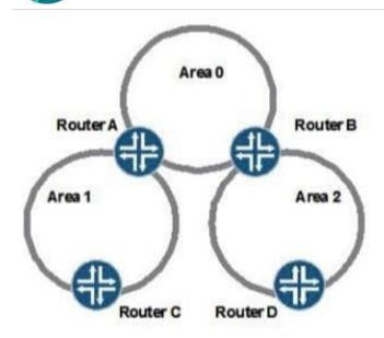
Given the OSPF network topology shown in the exhibit, you would like to inject external (non-OSPF) routes into the network on Router D.
