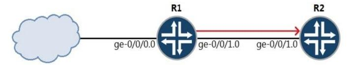
R1 assigns incoming voice traffic to the ef forwarding class. All other traffic is assigned to the best-effort forwarding class. You have configured a CoS re-write rule on R1 to include the correct CoS bit values in packets sent towards R2. You want R2 to classify traffic using the CoS markings created by R1.
