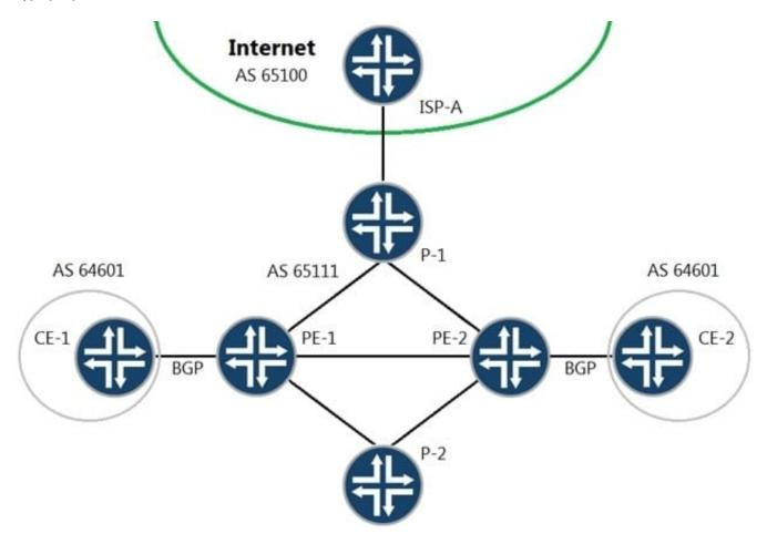
Referring to the exhibit, you have recently established a Layer 3 VPN between PE-1 and PE-2, connecting the two CE sites. Routing information is being shared between sites and the customer has two-way communication. After adding this VPN to your core network, PE-1 and PE-2 are no longer able to forward traffic to the Internet.
