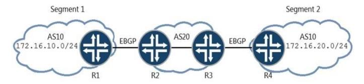
Your network connects two segments of your customer\\'s network as shown in the exhibit. They need to exchange routes between Segment 1 and Segment 2 but both segments use the same AS number.
