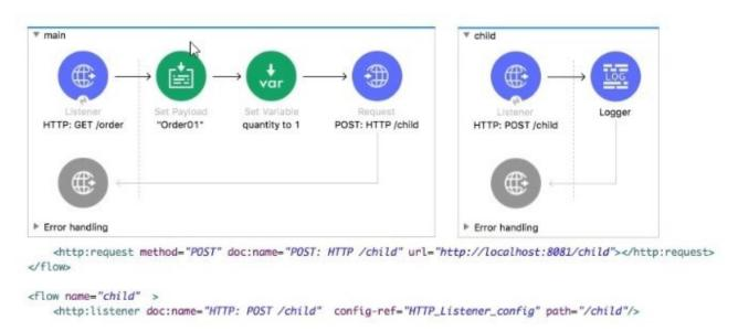
The main flow contains an HTTP Request. The HTTP Listeners and HTTP Request use default configurations.
