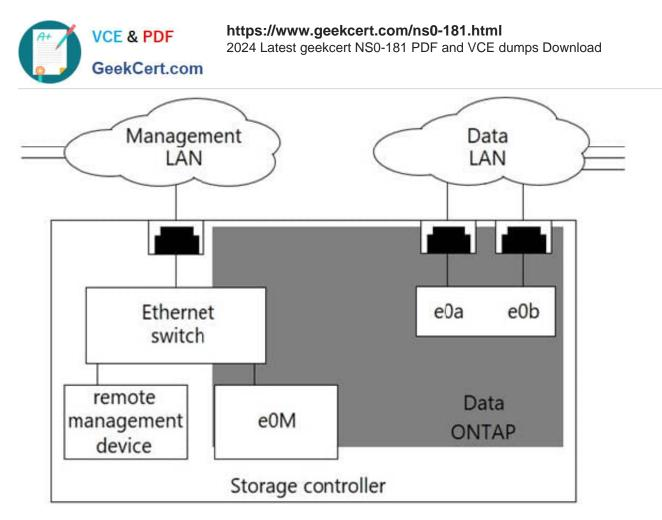
You are installing a new FAS cluster. The management network must be on tagged VLAN 11 for remote administration by a service provider. Referring to the exhibit, which two ports will allow service provider access to both cluster and node management LIFs? (Choose two.)
