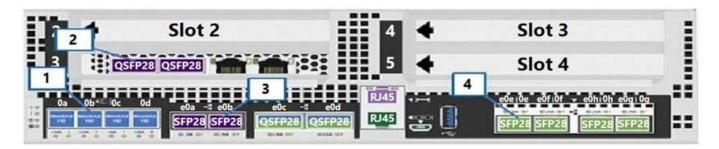
You are installing a 2-node AFF A400 switchless cluster. You have cabled the management network to the e0M port. NetApp also recommends cabling to a redundant management network switch.
