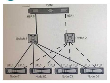
The host in the exhibit is connected to a 4-node ONTAP SAN using dual-fabric implementation. LUNs have been mapped LUN through all available UFs on nil (our nodes. Switch 2 is powered off for high- availability testing.
