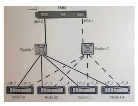
The host in the exhibit is connected to a 4-node ONTAP SAN using dual-fabric implementation. LUNs have been mapped LUN through all available UFs on nil (our nodes. Switch 2 is powered off for high- availability testing.
