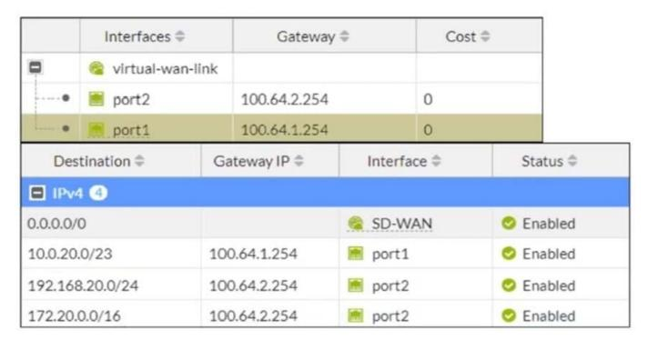
Exhibit A shows the SD-WAN performance SLA and exhibit B shows the SD-WAN member and the static routes configuration. If port2 is detected dead by FortiGate, which expected behavior is correct?
