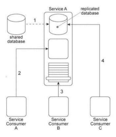
You\\'ve been told that the reason Service Consumers A and C bypass the published Service A service contract is because, for security reasons, they are not allowed to access a subset of the operations in the WSDL definition that expresses the service contract. How can the Service A architecture be changed to enforce these security restrictions while avoiding negative forms of coupling?
