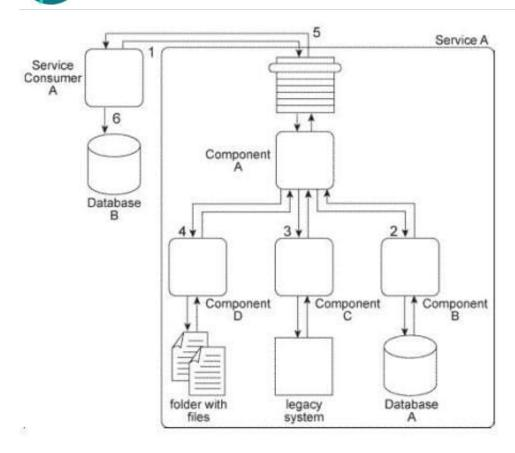
Service A is an entity service with a service architecture that has grown over the past few years. As a result of a service inventory-wide redesign project, you are asked to revisit the Service A service architecture in order to separate the logic provided by Components B, C, and D into three different utility services without disrupting the behavior of Service A as it relates to Service Consumer A. What steps can be taken to fulfill these requirements?
