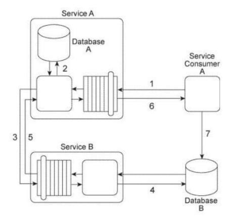
There are two problems with this service composition architecture that you are asked to address: First, both Service Consumer A and Service B need to transform the business document data from an XML format to a proprietary Comma Separated Value (CSV) in order to write the data to Database B. This has led to redundant data format transformation
