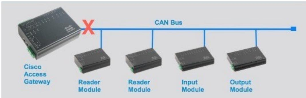
In the event of a loss of connectivity from the Cisco Access Gateway to the expansion modules on the CAN bus, with DC power still connected, what will happen if an access card was presented to a card reader that is connected to one of the Reader Modules?
